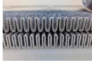
The Filter Media has absorbed water
