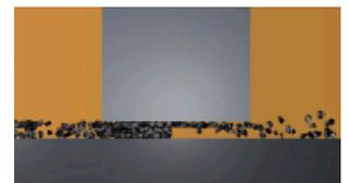
Solid contamination mainly causes surface damage and component wear.
