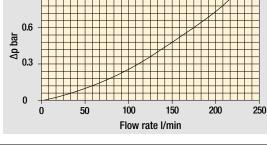
Bypass valve pressure drop
