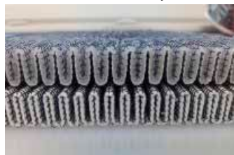
The Filter Media has absorbed water
