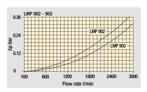
The curves are plotted using mineral oil with density of 0.86 kg/dm<sup>3</sup> in compliance with ISO 3968. ∆p varies proportionally with density.
