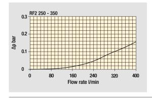
Bypass valve pressure drop
