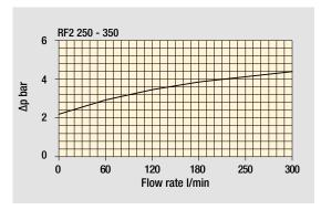
The curves are plotted using mineral oil with density of 0.86 kg/dm³ in compliance with ISO 3968. Δp varies proportionally with density.
