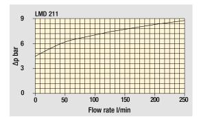
The curves are plotted using mineral oil with density of 0.86 kg/dm<sup>3</sup> in compliance with ISO 3968. Δp varies proportionally with density.
